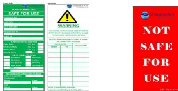
Figure 8. 2 Scaffold Safe For Use & Not Safe For Use tag
